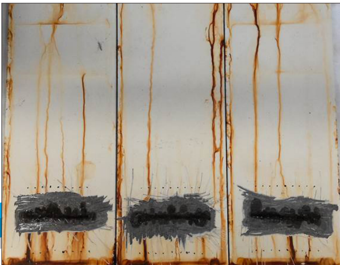
Traditional three-coat "passing" system in ISO 12944-9 CX.
