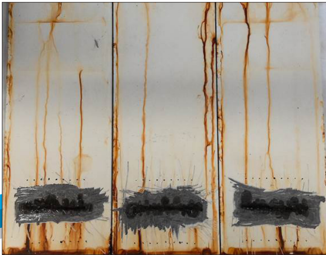
Traditional three-coat "passing" system in ISO 12944-9 CX.
