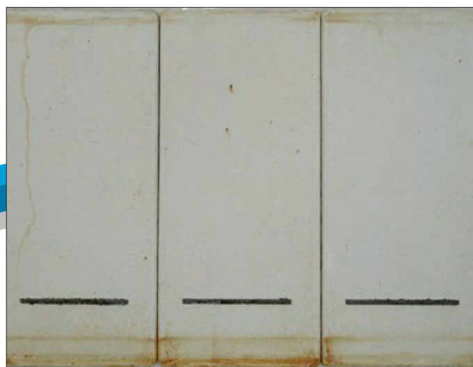
The new standard for corrosion protection: Armorlast passing 12944-9 CX four times
