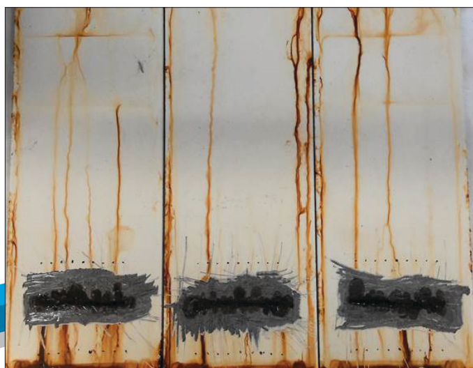
Traditional three-coat "passing" system in ISO 12944-9 CX.
