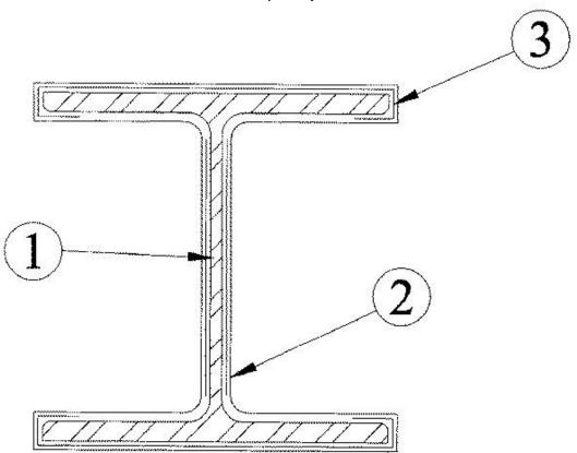
1. Steel Column — Min W10X49 wide flange steel column.
