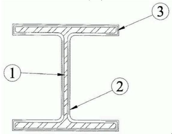
1. **Steel Column** — Min W10X49 wide flanged steel column. Hot dipped galvanized steel per ASTM A123. The column surfaces shall be prepared in accordance with the manufacturer's recommendations for galvanized steel and then primed with 3.5 mils of a cross-linked epoxy primer.
