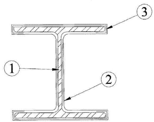
1. Steel Column — Wide flange steel columns having a W/D ratio of .84 to 3.55 and a maximum flange width of 16-1/8 in. See table in Item 2. Table not intended to be all inclusive.
