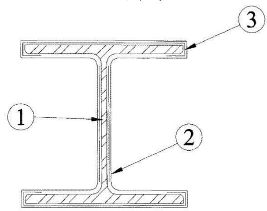
1. Steel Column — W14 x 342 wide flange steel column.
