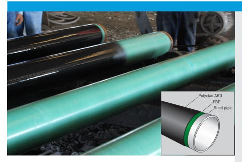
An advanced high performance coating formulated to protect Fusion Bonded Epoxy (FBE) coated buried steel pipe from damage during horizontal directional drilling installations.
