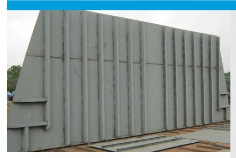
Carbozinc 8703 is a truly weldable inorganic zinc pre-construction primer formulated for shop application with very good spray and fast dry features for both hand and automated applications.
