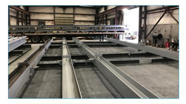
Structural steel members are shown in a laydown area following application of Carbocoat 8239 (Gray 0700) prior to delivery to a construction site in Tennessee. Fast-drying properties meant that beams could quickly be loaded onto trucks without the small laydown area running out of space and causing delays.
