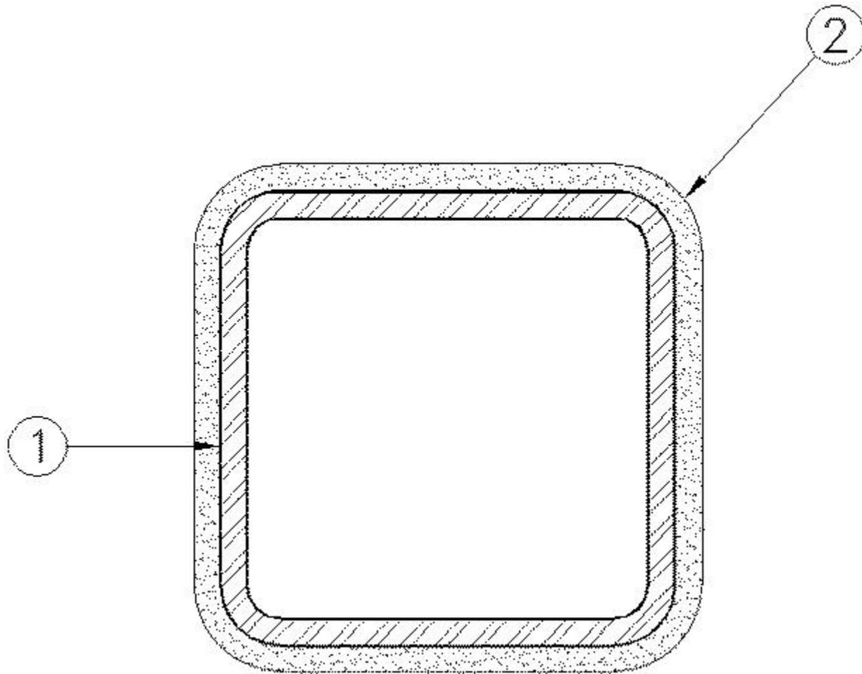
**1. Steel Column** — Square steel tube columns with the minimum sizes shown in the table below. Columns shall be free of dirt, loose scale and oil. Column shall be primed with metal alkyd primer.
