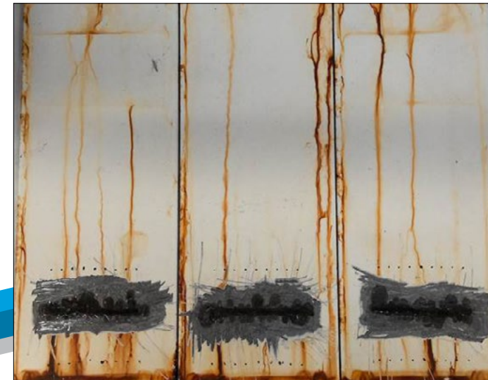
Traditional three-coat "passing" system in ISO 12944-9 CX.
