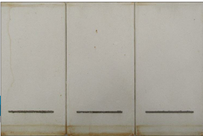
Armorlast panels after 12,600 hours ISO 12944-9 CX testing.
