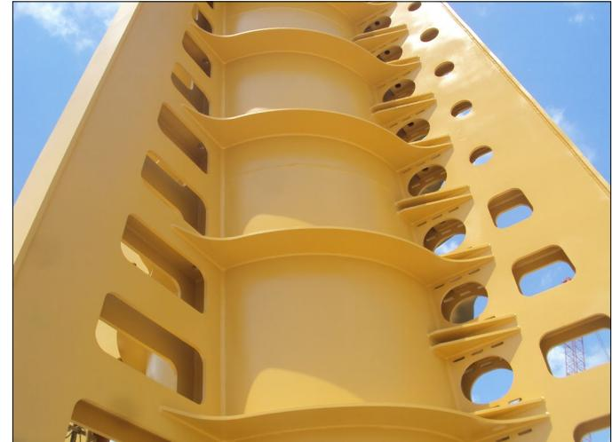
A lift boat leg tower is seen after application of Carbofleet 2635 as a finish coat.
