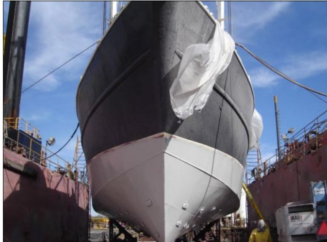
The hull of a trawler is seen after application of Carbofleet 2635 as the primer from the keel to water line. The high temperature that day was 35°F (1.7°C).
